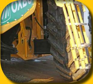
Sliding front axle: Tires and ladder slide in to allow for narrow transport width Optional Sliding rear axle: Both sides independently controlled within
