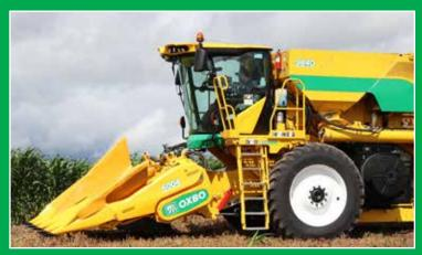
*Easy access cab:* Ladder retracts to keep width at a minimum
