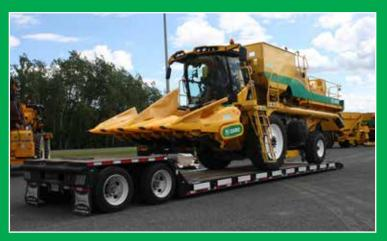
**Drive on for transport:** Axles slide in to narrow up combine to fit on standard trailer
