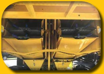
**Dual Sieve elements:** Makes fine tuning easy when harvesting different crops
