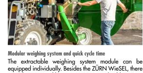
The extractable weighing system module can be equipped individually. Besides the ZÜRN WieSEL, there are other systems like HarvestMaster and Schlingmann available. Two turbines supply a strong airflow for high throughputs.
