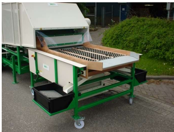
Pre-cleaner connected with a seed belt thresher
