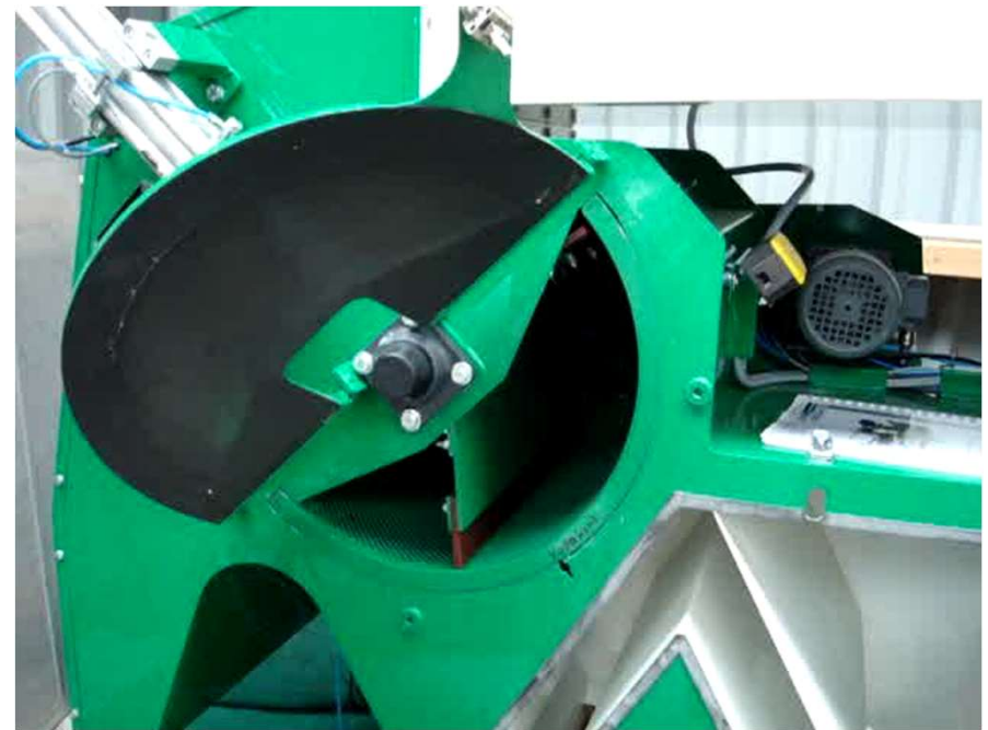
Pneumatic push out of threshing basket, for quick and easy inspection.
