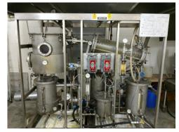
The Armfield FT29 is a self-contained, 25-liter batch process unit, that can extract 10 kilograms of oilseed per batch, and is ideal for producing a variety of solid/liquid extractions. Within each mode of operation of the FT29 unit, many
