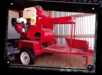
Large spike-tooth cylinder with grate concave and cleaning fan. Capacity with two people approximately one acre per day, depending on crop conditions. Heavy gauge metal construction, sealed, self-aligning bearings. Heavy duty trailer with leaf spring axle and 13" tires for towing.
