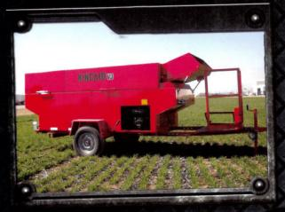
Gentle with seed, yet thorough threshing on most crops. Shaker shoe separation with air blast for final cleaning. Tension adjustments on pressure plates. Different screens available to accommodate wide range of seed sizes. Large rubber belts gently remove seeds for minimal seed damage and clean samples. Heavy steel construction, and sealed bearings. Coil spring axles and 14" tires.
