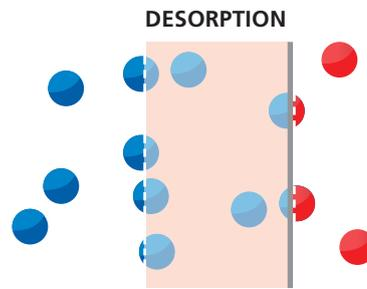
Adsorbate collects on the boundary surface and evaporates as gas
