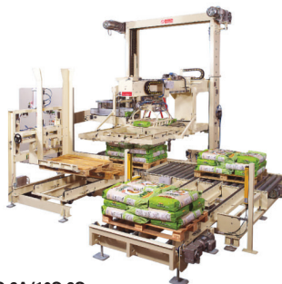
PS-3A/10S-2S Two column pick and place robot palletizer. Up to 750 bph
