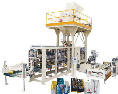
IMF high speed bagging line with double spout for preformed bags. Up to 1,800 bph ( 5-40 lbs 2-20 kg)
