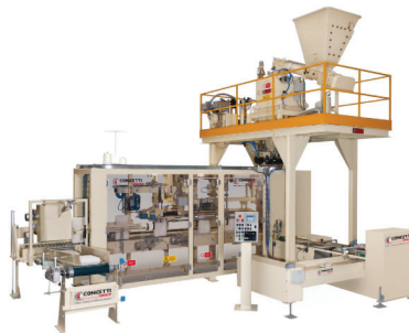
IGF fully automatic bag filler for preformed bags. Up to 1,200 bph (5-110 lbs 2-50 kg)
