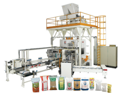
CAROUSEL equipped with six bagging stations. Fully automatic bag filler. Up to 1,200 bph with aerated products
